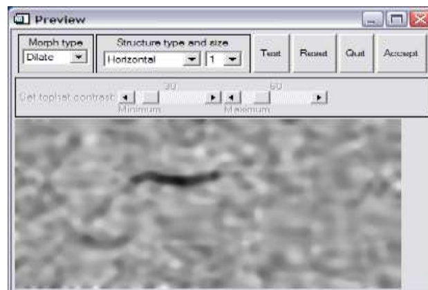
Figure 6: The Morphological filter interface providing a preview for a variety of combinations of filters with structuring element type and sizes.
